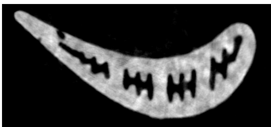
Neutron visualization of the blade of gas turbine engine
