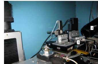
1 - sample 2 - first asymmetrical crystal, 3 - second asymmetric crystal, 4 - Detector
